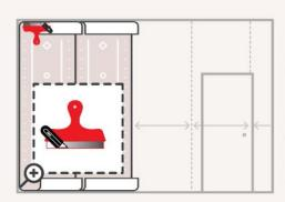
When you're happy with the position, using a straight edge, trim the excess wallpaper at the top and bottom of the wall. Use a sharp snap off blade knife. Push the paper into the ceiling line and skirting. Replace the blade often, as a dull blade can easily tear the wallpaper.
