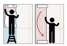
Attach the top of the length to the wall at the preferred height and in the correct position before letting go of the rest. Align the top and bottom of the first length before "smoothing down" the wallpaper. If you make a mistake, remove the length and start over. Apply more adhesive if the first coat has dried.
