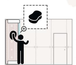
To get rid of air pockets, use a clean roller, sponge or brush, taking care not to squeeze out the paste between the joins and ensure the paste does not get onto the smoothing roller or sponge.
