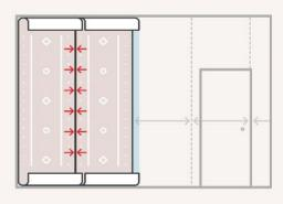
Butt join the lengths of wallpaper together, matching up the edges. Ensure that the lengths are properly positioned, that the pattern is matching and there is no surface visible at the joints. It is important that adhesive be applied right out to the edges to ensure the lengths adhere to the wall properly.
