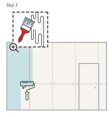
Our wallpapers are made using on a non-woven base, that means you apply the adhesive directly to the wall. Start by pasting an area sufficient enough to cover just over one drop width at a time. Use a paintbrush to cut-in around the areas too tight for the roller. (Such as at the ceiling line, corners, and along baseboards and trim).
