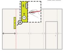
Put a mark close to the ceiling at this point. This is where you start your spirit-level or plumbline from and will allow half an inch overlap around the corner. Mark down the plumb-line every 11-15". This will give you a good vertical line to hang your first length to. Use Pencil Only.
