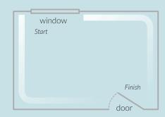
When installing wallpaper a good tip is to always work away from the main source of light and finish in the least conspicuous corner.
